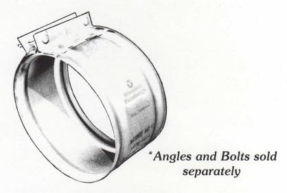
Strips rolled to fit your pipe. 2 ounce coated material meets AASHTO specifications. Bolt holes are in alignment with corrugations. O-ring gaskets available for all diameters.
